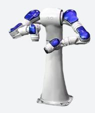
Suited for a variety of assembly applications, the 15-axis Motoman SDA10D dual arm robot provides human-like flexibility along with a slim design. The SDA10D offers a 10 kg payload per arm for outstanding performance. The Motoman SDA10D operates with either the DX100 or the NX100 controller which offer the ultimate in multiple axis control.
