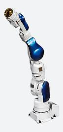
The Motoman SIA5D robot offers a low payload, high repeatability solution to assembly, injection molding, inspection, machine tending, packaging, and part transfer applications. This Motoman snake SIA5D DX100 robot accomplishes its tasks while taking up minimal space. Whether it's mounted on the floor, ceiling, wall, incline, or another machine, the SIA5D robot takes up as little as one square foot.
