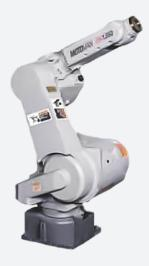
The Motoman DX1350 is used in part finishing applications such as material removal, sanding, and grinding. The rigid structure of the Motoman DX1350 XRC compact arm delivers high performance and accurate positioning. An IP67 rated wrist eliminates the need for a protective jacket on the Motoman DX1350 robot.
