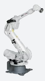
The Motoman HP165R is the shelf-mount version of the Motoman HP165. On shelf-mounted robots, such as Motoman HP 165R NX100, axis 2 is located further forward to increase the depth of the work envelope in a downward direction.
