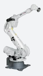
The Motoman HP165 sets the standard for versatility in the large robot market. This high-speed robot offers minimal footprint and superior performance in both spot welding and heavy payload handling applications.
