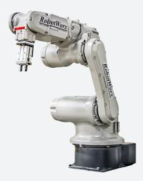
The Motoman HP3C is a compact robot perfect for small part applications such as assembly, dispensing, packaging, and material handling. Offering the widest work envelope in its class, and high-speed performance the HP3C NX100 is an ideal robot for any automation floor.
