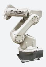
The compact Motoman HP3JC robot features a large work envelope and a payload of 3 kg. Multiple mounting options make it easy for the flexible HP3JC NXC100 to be integrated into any setting.
