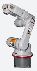
The Motoman HP3LC is the long arm version of the HP3C NX100 robot. With an extended reach of 859 mm, the HP3LC NX 100 offers the widest work envelope in its class.
