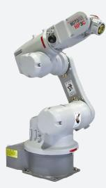
The Motoman HP3XF is an extra high-speed robot that requires minimal installation space. The S-Axis has a higher speed than the standard HP3 model. The HP3XF NX100 offers superior performance in small part applications such as assembly, dispensing, packaging, material handling, and machine tending.
