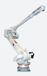
The Motoman HP50-20 is a dynamic, high-speed robot featuring an extended reach. This makes it ideal for processing large parts. It offers superior performance in arc welding, coating, dispensing, and material cutting applications. In many cell layouts, the HP50-20 NX100 robot has an extended reach eliminates the need for external axis tracks. This reduces the system cost and simplifies programming.
