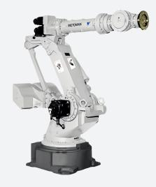
The high-performance, heavy payload Motoman HP 600 robot is a powerful addition to Motoman's extensive product line. The Motoman HP600 features parallel-link construction for strength, rigidity, and stabilization of high moment / inertia loads. Heavy-duty bearings provide smooth arm rotation. Its large payload is combined with a generous reach for versatility with extremely heavy loads.
