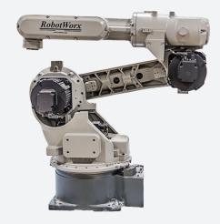
The Motoman HP 6RS is the short-arm, shelf mount variation. The Motoman HP6RS NX100 robot allows a larger work area because it has the ability to reach under and behind the robot body.
