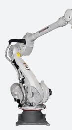
Part of the Expert Handling series, the Motoman EH200-150 features the longest reach and highest repeatability in its class. Specifically designed for heavy duty material handling applications, the EH200-150 NX100 robot's powerful design is ideal for any automation shop.
