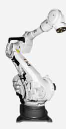
Part of the Expert Handling series, the Motoman EH200 sets a new standard in speed for large robots. It is designed for high-volume production applications such as material handling and machine tending. The EH200 uses the Motoman NX100 controller.
