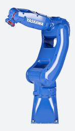
The Motoman GP8 is an advanced material handling robot that offers high speeds, an 8 kg payload, and 727 mm reach. There is only a single cable needed to connect the manipulator and controller, with an optional location for the manipulator cable connection which further helps to reduce interference with walls and also requires less installation space.
