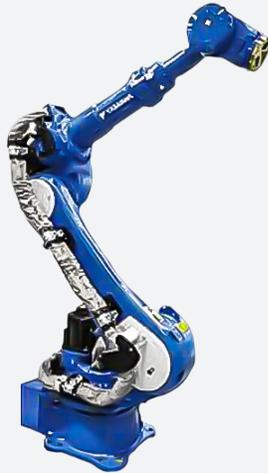
The floor mounted MH110 is a high payload and high moment and inertia ratings robot. It can handle larger and heavier payloads, up to 110 kg, and has a great reach at 2,236 mm horizontal reach and 3,751 mm vertical reach. The MH110 is a powerful six-axis robot that has fast motion speeds to help reduce cycle times and high-rigidity speed reducers.
