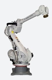
The versatile MH165-100 robot is fast, flexible, and powerful as it can tackle heavy payloads of up to 100 kg. It is a six-axis, floor mounted robot that has a large work envelope because of its reaches of 4,091 mm vertical, and 3,010 mm horizontal. The axial speeds are fast, helping to reduce cycle times and increase the overall output of production. Overall, the robot is slim which helps it reach into tight spaces, when necessary.
