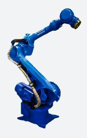
Yaskawa Motoman MH215 was developed as a large payload robot that not only excels at large product handling, but is also versatile enough for precision cutting and spot welding.
