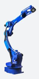
The 6-axis MH24-10 is a powerful (10 kg payload), high-speed robot that has very fast axis speeds and acceleration, all of which helps to reduce cycle times and increase output. It maintains a small footprint with its slim, yet contoured, arm design and extended reach of 2,010 mm. The reach and slim arm of the MH24-10 is ideal for agriculture, construction machinery, or automotive frames as it can access tight spots very easily.
