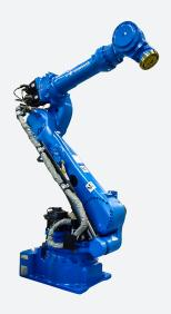
The Motoman MH250 robot can handle heavier parts and materials better than other robots in the Motoman MH series. This six-axis robot offers flexibility, even while handling materials weighing up to 250 kg. Maximum speed is just as fast as the lower payload MH robots. With its heavy payload, speed, and long reach, the Motoman MH250 DX100 robot generates faster production times and a more efficient process in material handling and parts transfer.
