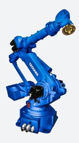
The versatile MH400 II is a high performance robot specifically used for heavy duty jobs as it can handle a payload up to 400 kg and multiple materials including ceramics, composites, metals, and polymers. The six-axis MH400 II has full capability with parallel link construction which boasts strength, rigidity, and stabilization for any loads bearing high moment or inertia.
