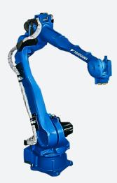
The Motoman MH50-35 industrial robot provides a much larger working envelope. While the payload capacity has been reduced, the MH50-35 DX100 still features a generous 35 kg payload and high-performance motors for maximum performance. There are used MH50-35 robots also available for sale. Every used Motoman MH50-35 has undergone a very meticulous refurbishment process and includes the RobotWorx Value Package.
