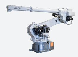
The high-speed Motoman MH50 is equipped with a long reach to easily handle large parts up to 50 kg. Optimized specifications improve robot performance for handling and cutting applications. The wide work envelope of the Motoman MH50 DX100 allows it to easily be integrated into a variety of situations.
