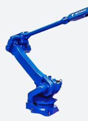
The powerful MH50II-20 is a high speed robot that is perfect for arc welding, coating, dispensing, material cutting, and handling applications. It's built on reliability and guaranteed to reduce cycle times as it has high-rigidity speed reducers paired with high-speed motion. In addition, the 20 kg payload and high inertia ratings make this robot the perfect solution for your heavy duty and large workloads.
