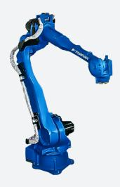
The powerful MH50 II-35 is a high speed robot that is perfect for coating, dispensing, material cutting, and handling applications because of its extended reach The six-axis MH50 II-35 is built on reliability and guaranteed to reduce cycle times as it has high-rigidity speed reducers paired with high-speed motion. In addition, the 35 kg payload and high inertia ratings make this robot the perfect solution for your heavy duty and large workloads.
