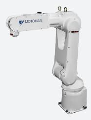
The Motoman MH5F is a compact robot featuring a 5 kg payload and uses minimal floorspace. This MH5F FS100 is great for many robotic applications including material handling, packaging, and assembly. The Motoman MH5F has internally routed cables and adjusts its performance based on the load.
