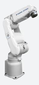
The Motoman MH5LS is a compact robot, ideal for arc welding, material handling, and assembly applications. The Motoman MH5LS has an extended reach of 895mm and is perfect for applications that require a larger work envelope. The MH5LS has internally routed cables that makes it safer and more reliable. Also availabe is the Motoman MH5LSM variant.
