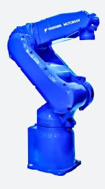
The Motoman MH5S has the widest work envelope in its class. With a 706mm reach and +/-0.02 mm repeatability, the Motoman MH5S offers high performance in material handling, assembly, machine tending, dispensing, and welding applications. The MH5S offers a 5 kg payload and has built-in collision avoidance that allows it to work together with up to 8 robots to produce the highest production performance.
