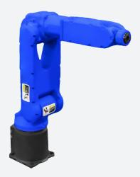
The Motoman MH5 robot arm is an economical solution to robot integration in small spaces. This powerful, compact MH5 robot arm offers a large work envelope and impressive 5 kg payload. It automatically adjusts for optimal performance based on payload requirements, even those less than 1 kg. The small footprint of the MH5 reduces installation requirements.
