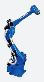
The Motoman MH80 industrial robot makes material handling, palletizing, and cutting applications easier than before. The MH80 material handling robot runs on DX100 controls and performs these industrial applications seamlessly. With the ability to palletize boxes and cases of different sizes, the MH80 DX100 industrial robot saves hundreds of hours and thousands of dollars.
