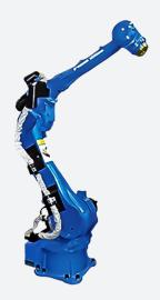
The MH80 II is a six-axis robot with a high wrist rating of IP67 that provides an increased handling capacity with a payload up to 80 kg. In addition, the MH80 II is very reliable, with its high-speed motion, high-rigidity speed reducers, and cables routed through the base and upper arm, all of which help to increase robot life and safety, while also reducing the cycle times.
