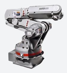
The Motoman K3 is a compact robot with a 3 kg payload and an MRC controller. It features a small footprint and fast cycle rates of 2.5m/s. The K3S can be floor, ceiling, or wall mounted. There are also used Motoman K3 robots available at RobotWorx. The experts at RobotWorx put all of their reconditioned robots through a meticulous refurbishment process, bringing them all back to like-new condition. Furthermore, any purchase of the used Motoman K3 robot will include the RobotWorx Value Package.
