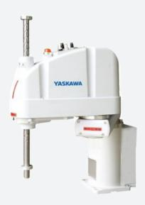
The Yaskawa Motoman MYS650LF SCARA robot will bring you superior performance to high-speed handling and assembly applications. This robot offers a 650 mm reach, a long (330 m) U-axis stroke, and a 6 kg maximum payload. The four-axis MYS650LF also brings high speeds in a very compact form that requires minimal mounting space. The high repeatability with compliance in all four axes make these robots ideal for assembly tasks.
