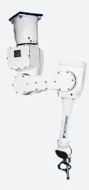
The Motoman MPK2F is a 5-axis, high performance robot. Ideal for high speed picking and packaging of food and consumer goods, the Motoman MPK2F is sure to increase your production. The Motoman MPK2F has a 2 kg payload, 900 mm horizontal reach, and comes with the advanced FS100 controller.
