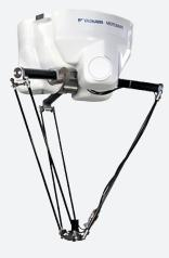
The Motoman MPP3 is a high speed pick and place robot that has zero footprint! You can optimize space with its compact design. The MPP3 is easy to clean due to its seamless covers.
