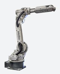
Motoman SSF2000 is a compact robot that features a 6kg payload and the widest working envelope in its class. With built-in collision avoidance and the ability to cut cycle time by fifteen percent, the SSF2000 NX100 robot is ideal for maximum productivity.
