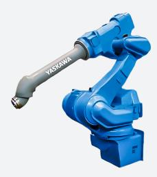
Motoman's EPX2800R robot is a shelf-mounted robot that offers many of the same advantages as other Motoman painting robots. The robot is still designed with six axes, but an optional seventh axis can be added for rail-mounting. A longer reach of 2,825 mm also differentiates this robot from others in Motoman's EPX series. The Motoman EPX2800R NX100 robot's 15 kg maximum payload capacity, 2.0 m/s maximum speed, and shelf-mount style make coating and dispensing applications easy and efficient.
