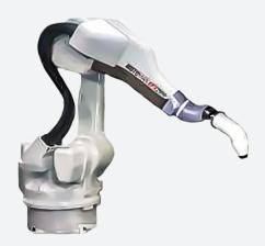
The Motoman EPX2900 completes painting applications with a smooth and consistent finish. Offering a large work envelope the versatile EPX2900 NX100 is ideal for use in automotive factories, painting agricultural equipment and other machinery and large parts.
