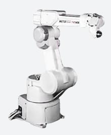
Motoman's high-speed PX1450 robot is available with either a three-roll or Lemma-style wrist, providing versatility and a smooth, superior performance in standard industrial and automotive coating applications. The three-roll wrist design is ideal for painting contoured parts such as car bodies and interior/exterior surfaces. The Lemma wrist is well-suited for painting horizontal and vertical planes.
