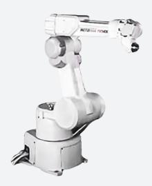
The high-speed Motoman PX1850 robot is available with either a three-roll or Lemma-style wrist, providing versatility and a smooth, superior performance in standard industrial and automotive coating applications. The three-roll wrist design is ideal for painting contoured parts such as car bodies and interior/exterior surfaces. The Lemma wrist is well-suited for painting horizontal and vertical planes.
