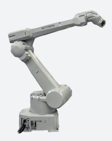
The Motoman PX2850 robot is available with either a three-roll or hollow style wrist, providing versatility and superior performance in standard industrial and automotive painting applications. The three-roll wrist design is ideal for painting contoured parts such as car bodies and interior/exterior surfaces.
