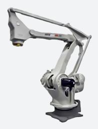
The extensive vertical reach on the Motoman MPL300 helps reduce cycle times during palletizing applications. Features such as pallet handling, layer handling, and the optional EasyPallet Pendant make the MPL300 DX100/MPL200 an excellent choice to improve the palletizing process.
