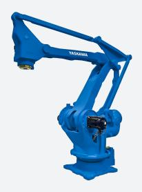
The versatile MPL300 II is a 4-axis, high performance robot that has a payload of 300 kg, extensive reach of 3,024 mm vertical, 3,159 mm horizontal reach, and a ±0.5 mm repeatability. This reach allows the MPL300 II to build loads up to 102 inches tall with standard 48 in. x 40 in. pallets. It is the perfect robot to handle numerous palletizing jobs such as case palletizing, bag palletizing, de-palletizing, layer forming, and layer picking.
