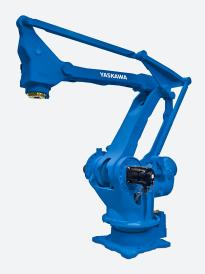
Increasing production through faster and more reliable automation methods are key reasons to consider the Motoman MPL800. It stands out with its ability to handle 500 kg loads up to 3024 mm away. The MPL800 DX100 is a four-axis dedicated pelletizing machine that can service multiple infeed conveyors and up to four pallet build locations.
