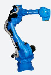
For palletizing applications that need to handle up to 80 kg, the Motoman MPL80 is an ideal choice. With fast axis speeds and high acceleration, this robot arm, new or used, can increase throughput and maximize production. Precise movements and a wide 360 degree work envelope allow this arm to accurately service multiple infeed conveyors and up to two pallet build locations.
