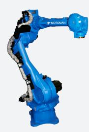
The Motoman MPL80 II is the advanced palletizing robot that comes equipped with the DX200 controller. The Motoman MPL80 II has 5 controlled axes and can handle an 80 kg payload. Versatile in its palletizing abilities, the MPL80 II can perform case palletizing, bag palletizing, order picking, and more. It has an upgraded design with internally routed cables to create maximum reliability, and has a compact base to reduce footprint.
