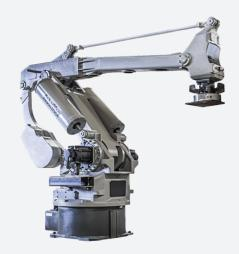
The high speed Motoman SP100 is a four-axis palletizing robot capable of handling high payloads. Palletizing robots are ideal for applications that require repetitive, continuous movement of heavy loads. An expanded work area and increased speed allow the SP100 to service multiple infeed conveyors or pallet stations.
