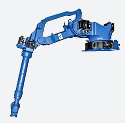
The high-speed EPH130RLD offers a 3,474 mm horizontal reach; 4,151 mm vertical; and  $\pm 0.3$ mm repeatability. These specs allow improved clearance for die changes and give enough spacing (from 4-7 m) when used for press tending. In addition, there is a high vibration rating making it ideal for the press room.
