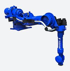
The six-axis ES165RD II is a high-speed, shelf-mounted robot that is designed for optimal performance for heavy loads (up to 165kg) and machine/press tending applications. The cable and air lines will have a longer life as they are routed through the robot base to the upper arm. This design, and the Functional Safety Unit integrated into the DX200 controller, are key safety features.
