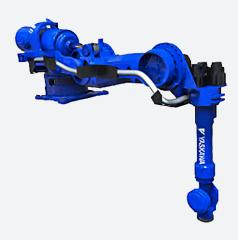
The six-axis ES200RD II is a high-speed, shelf-mounted robot that is designed for optimal performance for heavy loads (up to 200 kg) and machine/press tending applications. The cable and air lines will have a longer life as they are routed through the robot base to the upper arm. This design, and the Functional Safety Unit integrated into the DX200 controller, are key safety features.
